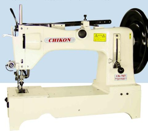
This machine is equipped with semi-rotary large capacity shuttle hook, suitable for sewing extra heavy weight materials such as safety and logging belts, luggage, cargo slings, buffing wheels, harnesses, construction barriers, parachutes, balloons and book binding.
