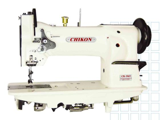
This machine is equipped with unison feed mechanism and vertical-axis double-capacity hook. It is applicable to an extended range of heavy materials for industrial use, such as cargo handling belts and containers, as well as those for general use, such as car seats, sofas and bags, etc.
