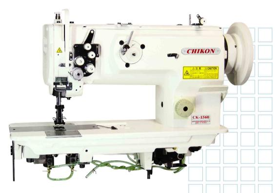
This machine is equipped with unison feed mechanism and vertical-axis double-capacity hook. It is applicable to an extended range of heavy materials for industrial use, such as cargo handling belts and containers, as well as those for general use, such as car seats, sofas and bags, etc.
