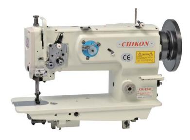
1-needle, Unison-feed, Lockstitch Machine with Horizontal-axis Large Hook
